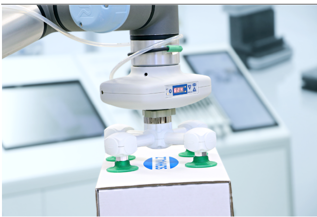
Pneumatic vacuum generator RECB when handling cardboard boxes
